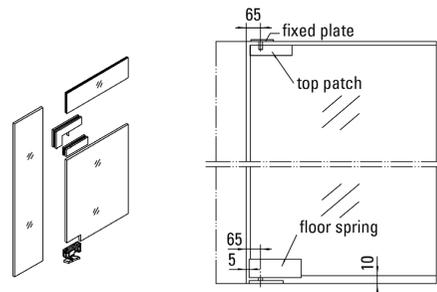
When used with top patch or top pivot, pivot center must be aligned with floor spring pivot center.
