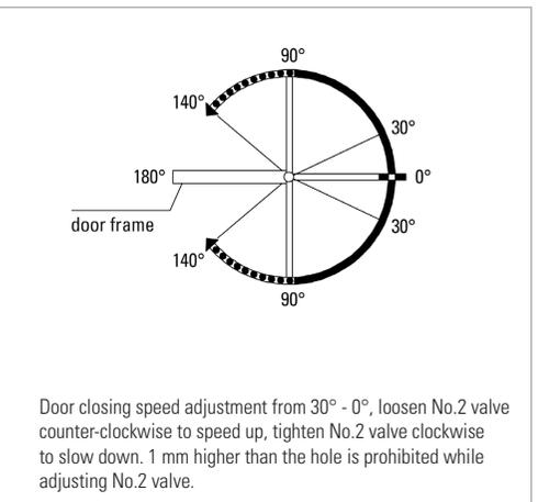
Door closing speed adjustment from 30° - 0°, loosen No.2 valve counter-clockwise to speed up, tighten No.2 valve clockwise to slow down. 1 mm higher than the hole is prohibited while adjusting No.2 valve.
