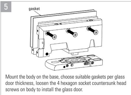
Mount the body on the base, choose suitable gaskets per glass door thickness, loosen the 4 hexagon socket countersunk head screws on body to install the glass door.
