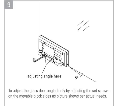
To adjust the glass door angle finely by adjusting the set screws on the movable block sides as picture shows per actual needs.
