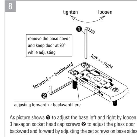
As picture shows ❶ to adjust the base left and right by loosen 3 hexagon socket head cap screws ❷ to adjust the glass door backward and forward by adjusting the set screws on base sides.
