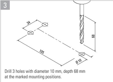
Drill 3 holes with diameter 10 mm, depth 68 mm at the marked mounting positions.
