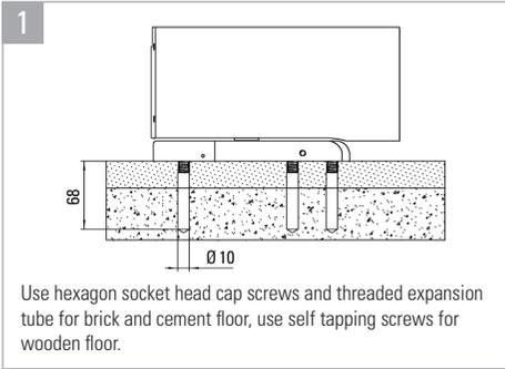
Use hexagon socket head cap screws and threaded expansion tube for brick and cement floor, use self tapping screws for wooden floor.
