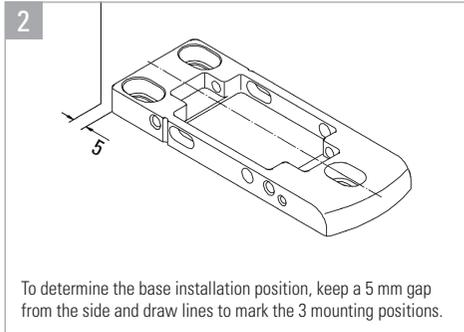
To determine the base installation position, keep a 5 mm gap from the side and draw lines to mark the 3 mounting positions.
