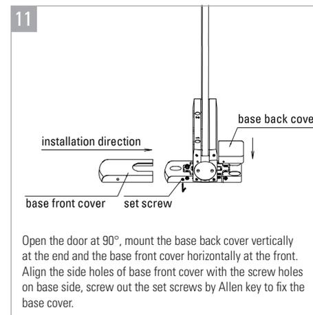
Open the door at 90°, mount the base back cover vertically at the end and the base front cover horizontally at the front. Align the side holes of base front cover with the screw holes on base side, screw out the set screws by Allen key to fix the base cover.
