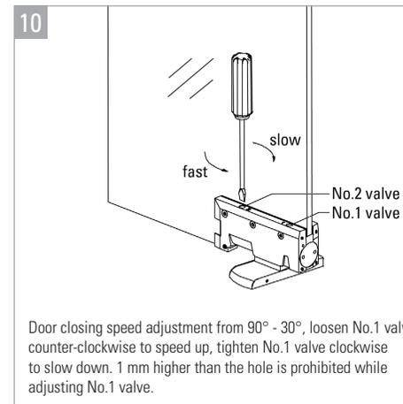
Door closing speed adjustment from 90° - 30°, loosen No.1 valve counter-clockwise to speed up, tighten No.1 valve clockwise to slow down. 1 mm higher than the hole is prohibited while adjusting No.1 valve.
