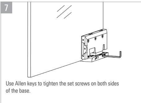
Use Allen keys to tighten the set screws on both sides of the base.
