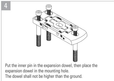
Put the inner pin in the expansion dowel, then place the expansion dowel in the mounting hole. The dowel shall not be higher than the ground.
