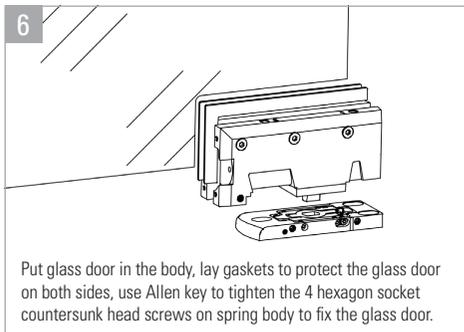
Put glass door in the body, lay gaskets to protect the glass door on both sides, use Allen key to tighten the 4 hexagon socket countersunk head screws on spring body to fix the glass door.
